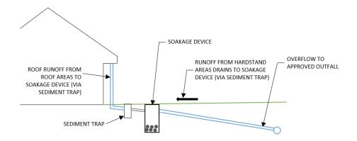
Figure 3: Schematic showing typical arrangement for soakage reduced
